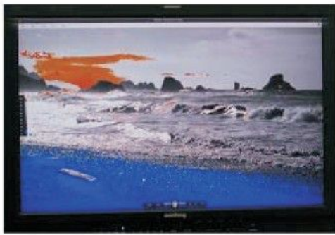
LUM Coloring In Default Mode. Color Coded Regions: Upper 90-100 IRE Lower 0-10IRE
