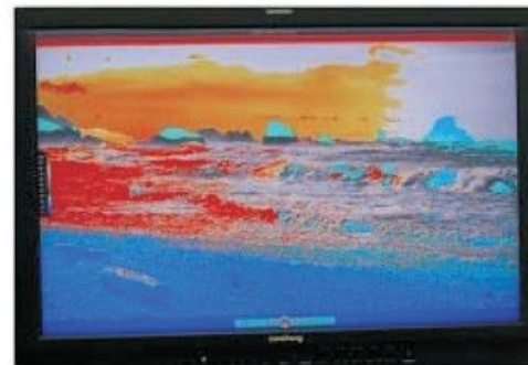
LUM Coloring with Color Coded Regions set to: Upper > 70 IRE Lower < 40 IRE. 40 to 70 IRE shown as gray scale.
