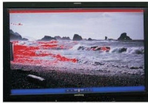
LUM Coloring With Color Coded Regions set to: Upper > 100IRE Lower < 0 IRE
